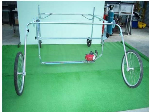
position from the rear ensuring the fingers are positioned across the machine in roughly the correct position. Ensure lift lever is vertical. Fit the support tube on the spigot at the left hand side and secure the right hand end in position with the triknob
