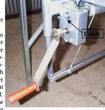
weight (sandbag) may need adding to the winch frame at end opposite winch to achieve this. If binding of the system occurs, check main frame is levelled and there is no frame twisting.
