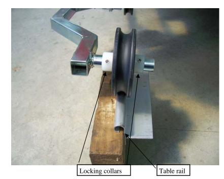
the locating collars and move the wheels sideways until the harvester sits correctly on the table rails. Move the collars to within 1mm of the wheels and lock in place.
