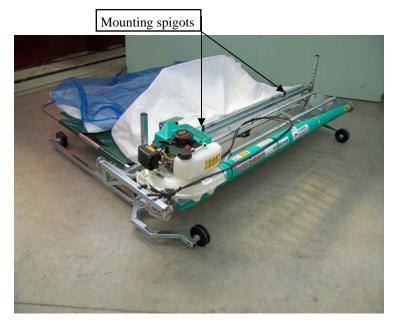
should already be fitted to the quick release frame. Lift up by the steel frame and position it over the 2 mounting spigots
