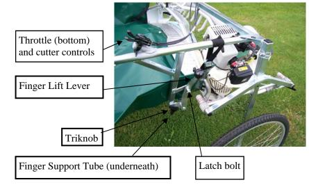
8. With the finger clamp screws undone, move the fingers side ways to suit the row width being cut. As a rough guide the finger width should be similar to the pruned width of the plant being harvested. The clamps are also lift travel stops—see below:-
