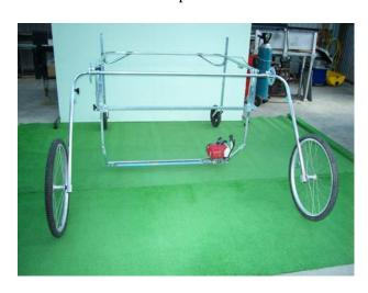
position from the rear ensuring the fingers are positioned across the machine in roughly the correct position. Ensure lift lever is vertical. Fit the support tube on the spigot at the left hand side and secure the right hand end in position with the triknob
